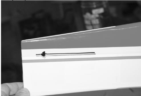
13. Insert the elevator into the slot in the rear fuselage side. It must be inserted upside down with the counter balances facing the rear of the plane, then it can be noted into the grant position. Places are all staffer detail.
