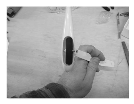
8. Open the gear slots in the side of the fuselage with a sharp hobby knife.
