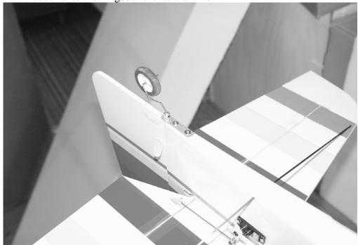
21. Secure the rudder hinges with thin CA
