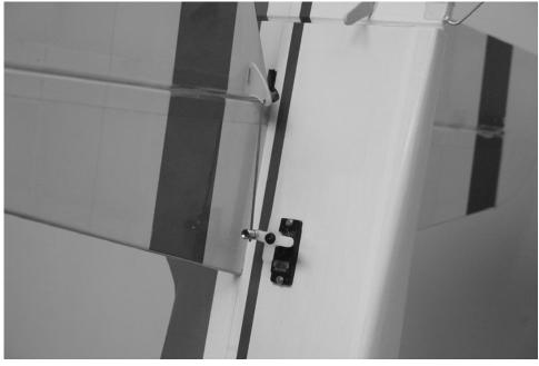
26. Locate the (2) .060 carbon fiber reinforcement rods. Use a drill bit with a pen vise to open holes in the outer leading edge of the stab and in the solid wood part of the bottom rear of the fuselage as shown.
