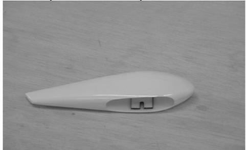
6. Make a slot in the wheel pant using the slot in the ply plate as a guide. It should be big enough to slide over the threaded portion of the axle.
