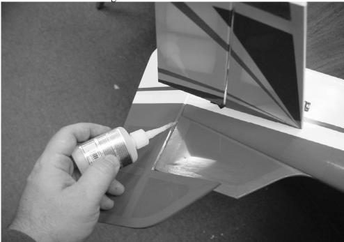
22. Locate the elevator control horn. Use a sharp hobby knife to remove the
