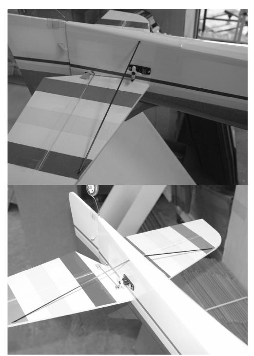
28. Use a #11 blade to remove the covering from the slot near the bottom of the rudder. Locate the composite control horn for the rudder. Scuff the control horn to remove the glossy finish and glue into place in the slot in the rudder. Be sure to center the horn in the slot.
