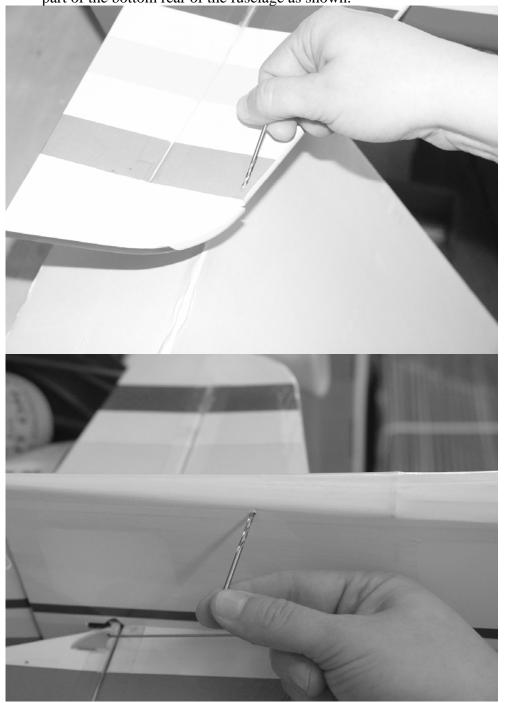
27. Use medium CA or epoxy to secure the rods into position as shown in the photos. Make sure alignment is correct before gluing. DO NOT OMIT THESE REINFORCEMENTS!!!
