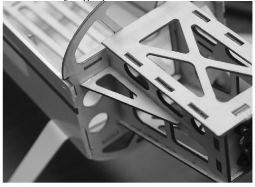
12. Open the horizontal stabilizer mounting slot in the rear of the fuselage with a
