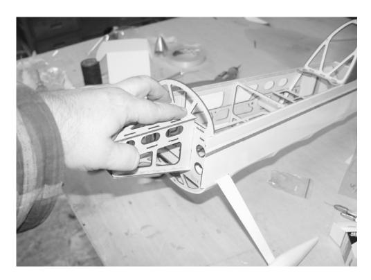
11. Add the 2 triangle support pieces to the motor box and secure with medium CA.
